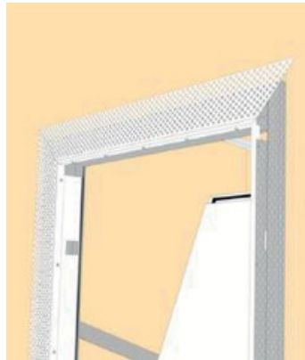
Skimmed finish and damper panel can then both be painted to match.
